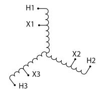
Three Phase Encapsulated Autotransformer with a capacity of 75kVA, transforming 600Y Volts to 480Y Volts
