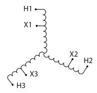
Three Phase Encapsulated Autotransformer with a capacity of 300kVA, transforming 600Y Volts to 480Y Volts
